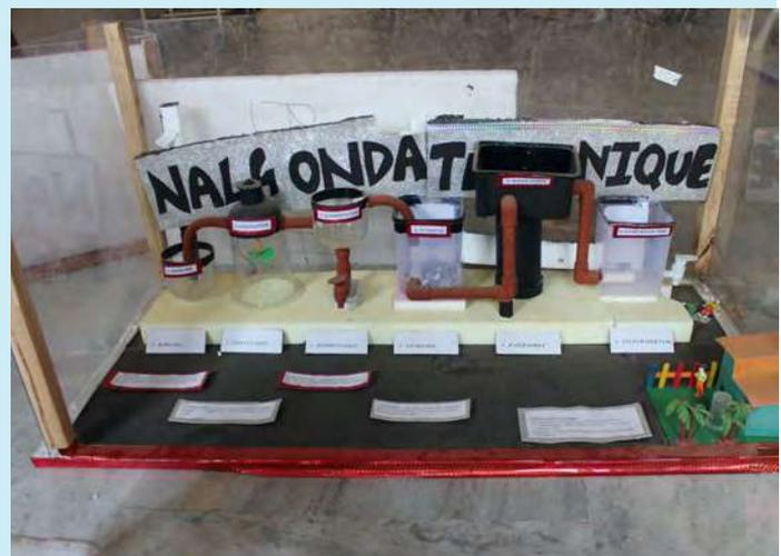
National Environmental Engineering Research Institute (NEERI), Nagpur has evolved an economical and simple method for removal of fluoride which is referred to as “Nalgonda Technique” (Nawlakhe et al 1974). The process comprises addition in sequence of sodium aluminate (filter alum), lime and bleaching powder to the fluoride water followed by flocculation, sedimentation and filtration. This technique is extremely useful for both domestic as well as for community water supply.
