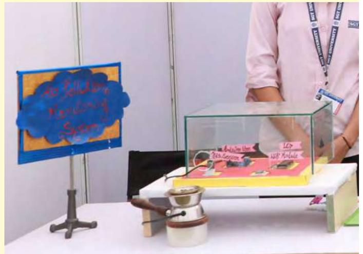
It monitors the Air Quality over a web server using internet and triggers an alarm when the air quality goes down beyond a certain level, means when there are sufficient amount of harmful gases present in the air. It shows the air quality in PPM on the LCD and as well as on webpage so that we can monitor it very easily. In this IOT project, you can monitor the pollution level using your computer or mobile using wi-fi module.
