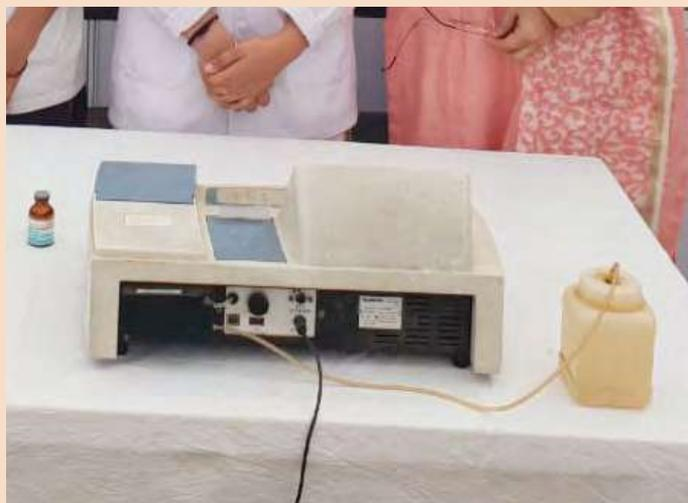
Chemistry analyzers are used to determine the concentration of certain metabolites, electrolytes, proteins, and enzymes in the samples of serum, plasma, urine, cerebrospinal fluid and other body fluids. Biochemical tests can be used for screening of disease, for confirmation of a diagnosis made on clinical examination, for monitoring the progression of a disease and outcome of the treatment.
