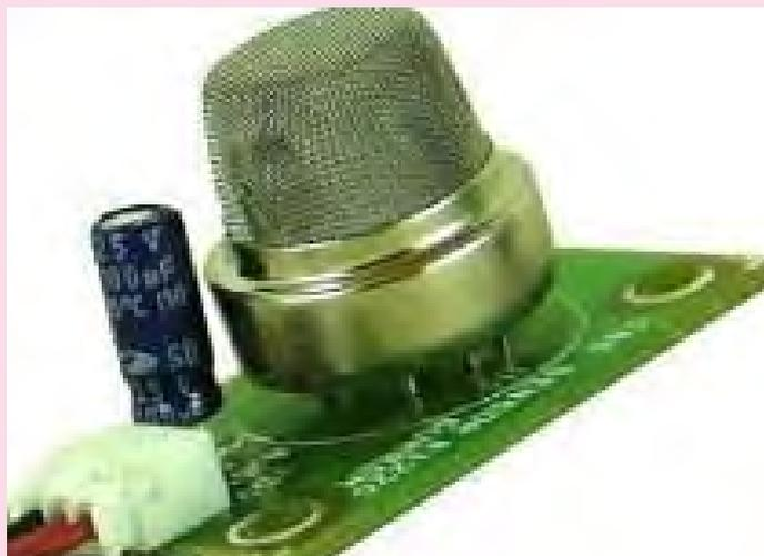
This type of device is important because there are many gases that can be harmful to organic life, such as humans or animals. Gas detectors can be used to detect combustible, flammable and toxic gases, and oxygen depletion. Gas leak detection is the process of identifying potentially hazardous gas leaks by sensors.
